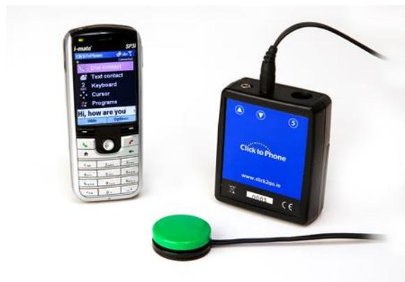
**The Click-to-Phone enables a person who cannot press the keys of a mobile phone to operate the phone with a single switch, a 5 switch device or the joystick on their powered wheelchair.**
